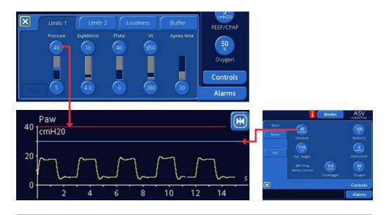
Check that the high Pressure alarm limit is set to an appropriate value. Suggestions: Normal patient: 40 cmH<sub>2</sub>O for 100% MinVol
