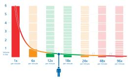
Optimal combination of tidal volume / respiratory rate (in this example 15 x 400 ml for a minute volume of 6l)
